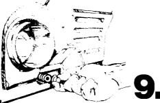
Remove the red cap from the the gas pipe. Move the dryer into its final position
